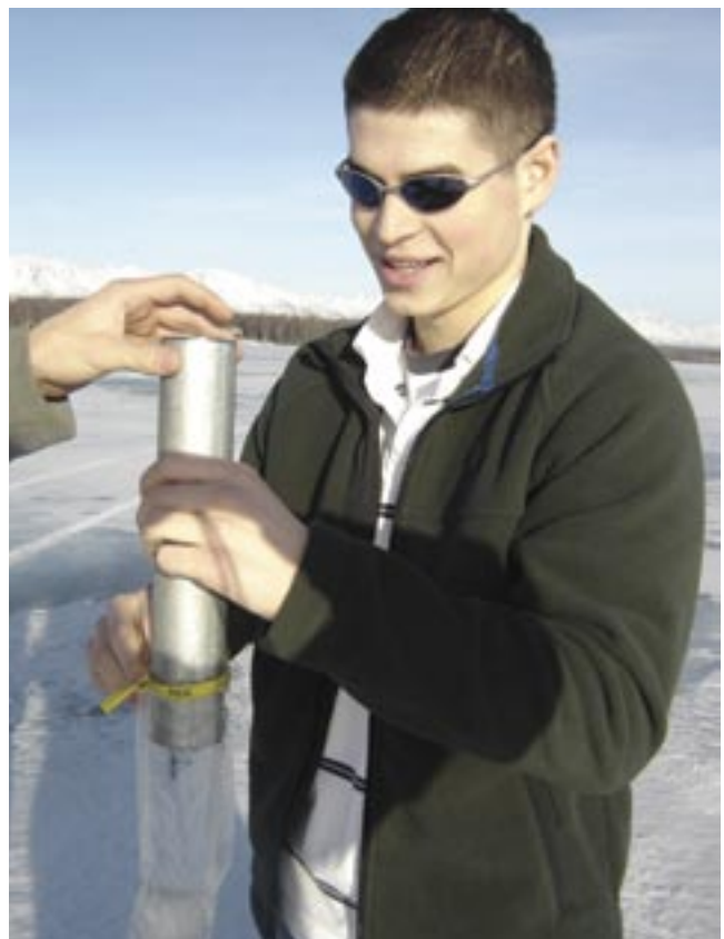
(Above) A snow sampling tube of known cross-sectional area is used to obtain three snow samples. (Opposite) A hot-wire gauge is used to measure ice thickness. Safety note: Students and teachers must take extreme care when walking on ice.
