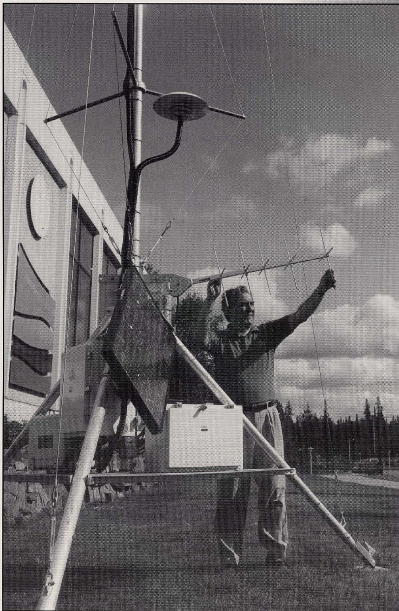
NEW-NET — Professor Glenn Shaw adjusts an arm of a new radiation monitoring device set up in front of the institute this summer. Radiation levels in the surrounding area are instantly displayed on a digital panel attached to the instrument.
