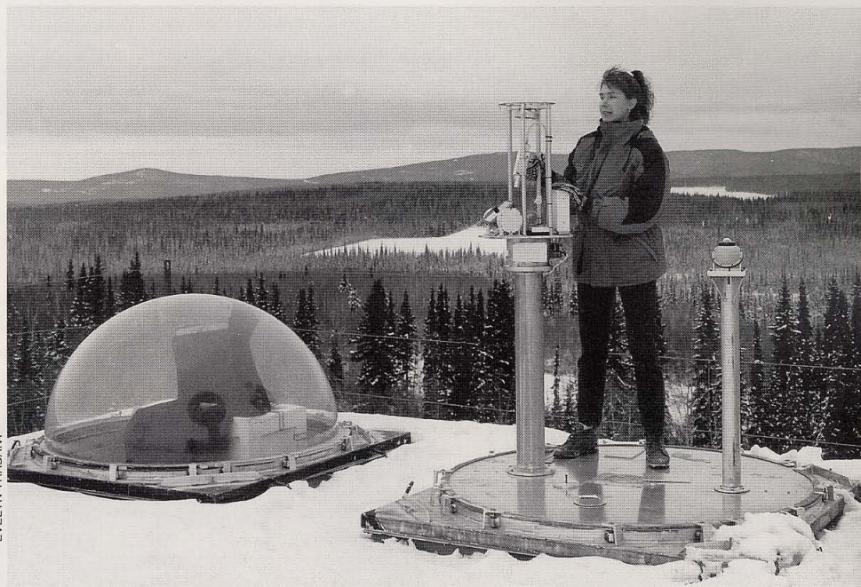
Climate Check —Graduate student Tove Svendby checks a solar tracker used to measure atmospheric gas from the Geophysical Institute roof. A similar instrument will be housed in a new Climate Change Monitoring Station this spring.
