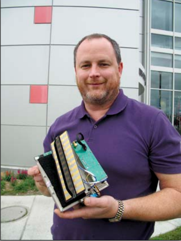
INSTRUMENT —Poker Flat Research Range Manager Greg Walker holds a synthetic aperture radar unit that will fit in the nose of an unmanned aircraft. Photo by Ned Rozzell.
