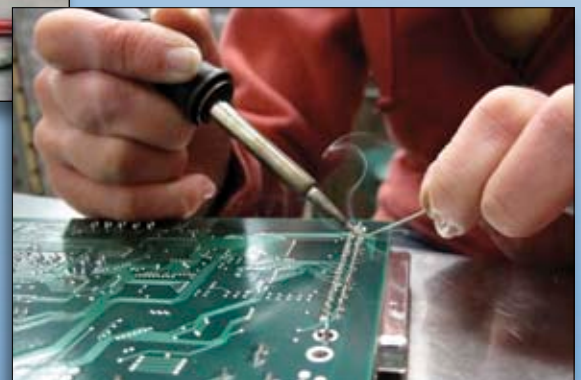
CIRCUITRY —Above and right, Gwen Bryson solders a component on a circuit board for a new SuperDARN system recently installed in Antarctica. Bryson is now employed with the Alaska Satellite Facility. Photos by Ned Rozell.
