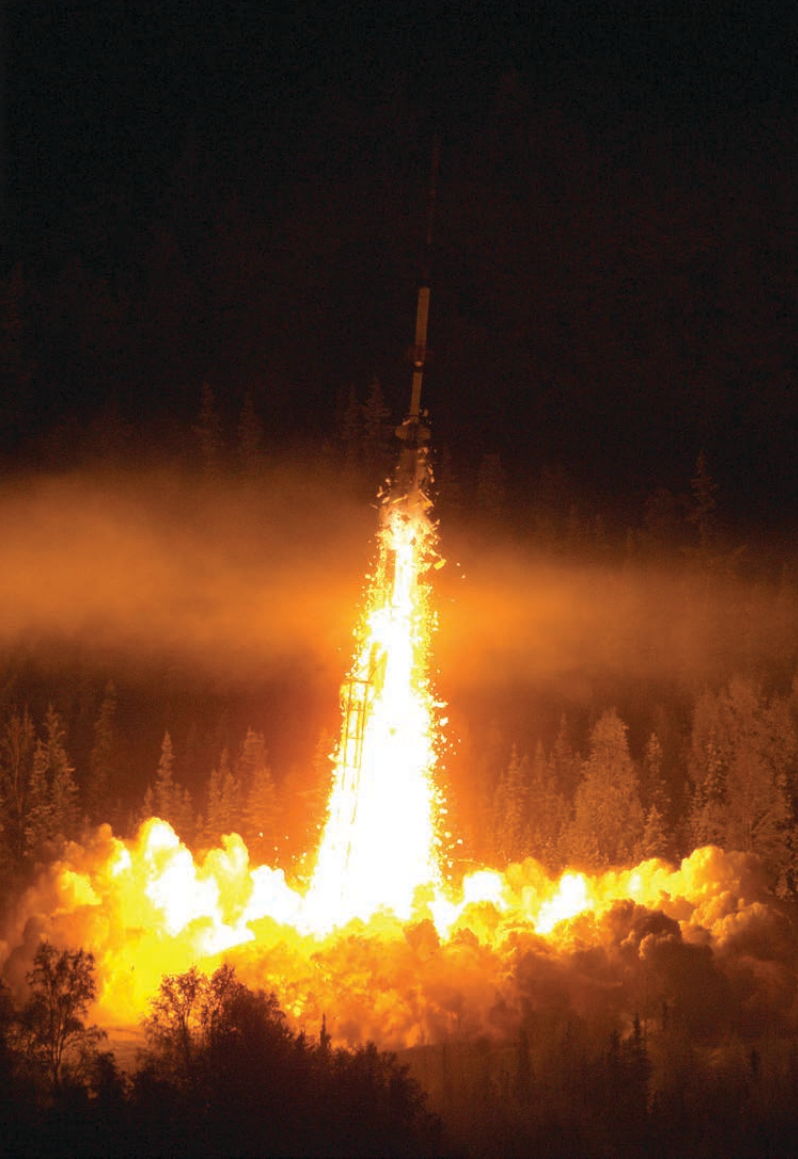
LAUNCH —Left: Bits of styrofoam fly off the rocket as it launches. Styrofoam is used before launch to keep the solid fuel in the rocket motors from freezing, which could damage them. Photo by Lee Wingfield, NASA. Right: A composite photo showing all four rockets launched on January 26. The stars are wheeling in the sky in this long exposure, and the white clouds of TMA are visible. Photo by Jamie Lee Adkins, NASA.
