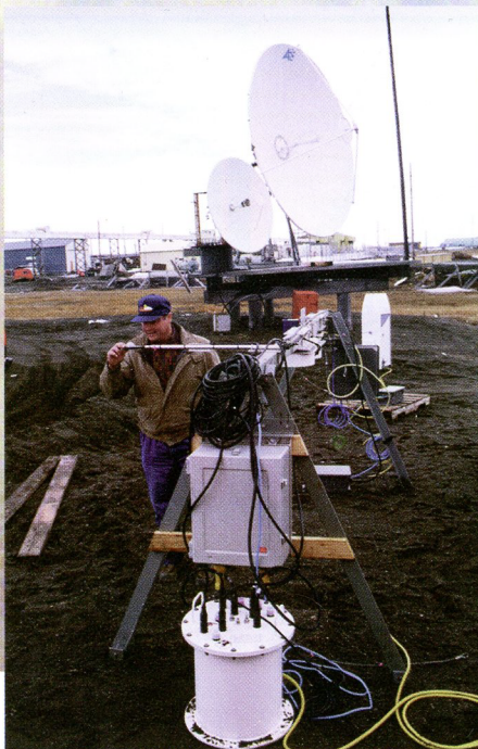
At left, Utley checks an array of instruments that measures radiation downwelling from the sky. Above, he adjusts instruments that measure reflected light and infrared radiation upwelling from the ground.
