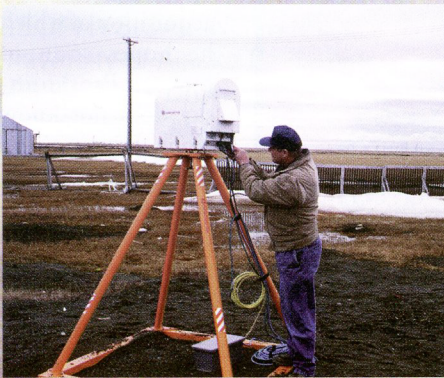
Above, ARM Instrument Specialist Phil Utley inspects a microwave radiometer, which measures water vapor and cloud water present in a column extending from above the instrument to the top of Earth's atmosphere.
