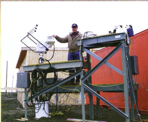
Above, ARM Instrument Specialist Phil Utley inspects a microwave radiometer, which measures water vapor and cloud water present in a column extending from above the instrument to the top of Earth's atmosphere.
